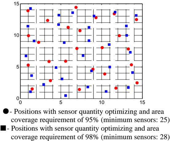
Figure 4. Minimum sensor nodes deployment in 225 grids
