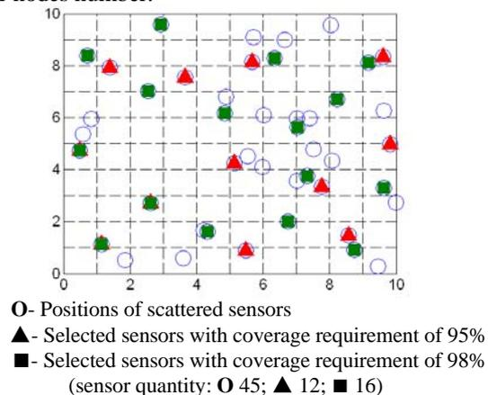
Figure 5. Simulation result of random sensor nodes deployment
