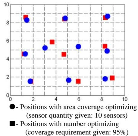
Figure 3. Sensor nodes deployment in 100 grids
