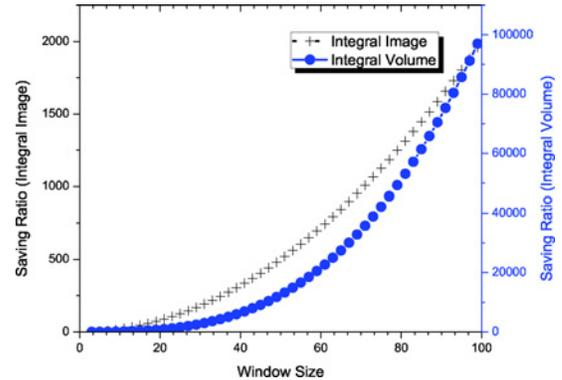
Fig. 6. Analysis of computational efficiency for focus measure computation using integral space.
