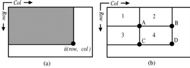
Fig. 2. Image integral to (a) calculate rectangular area (shaded), (b) compute sum of pixels within sub-window 4.
