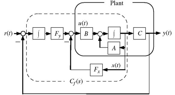
Figure 1. State feedback integral controller for delay-free plant.
