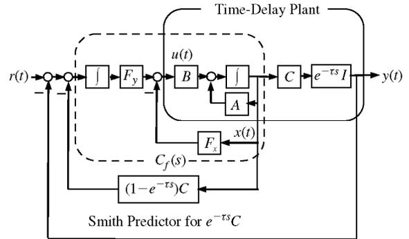
Figure 2. State feedback integral controller with the Smith predictor for  $e^{-\tau s}C$ .
