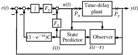
Figure 3. Output feedback integral controller for time-delay plant.
