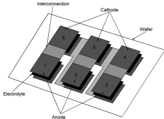
**Figure 16.** The schematic of lateral configuration of the micro SOFC stack.
