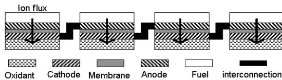
**Figure 14.** Banded planar interconnection for the fuel cell stack.
