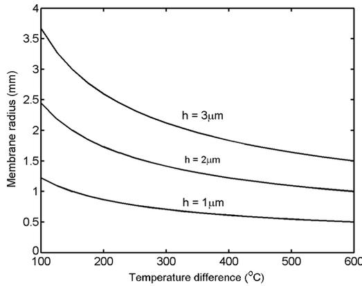
**Figure 4.** The maximum membrane radius versus temperature difference for a corrugated YSZ film ( $H:h = 10$ ,  $\beta = 5$ ).
