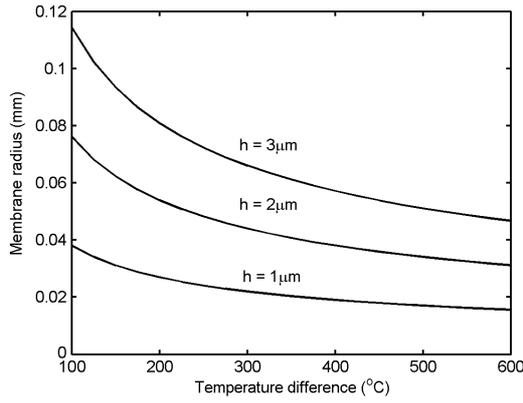
**Figure 3.** The maximum membrane radius versus temperature difference for a flat YSZ film.
