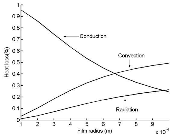
**Figure 12.** Heat loss versus film radius at the temperature difference of 350 K.
