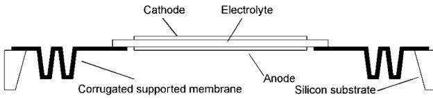
**Figure 9.** A flat thin electrolyte film mounted on a corrugated supporting membrane.
