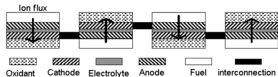
**Figure 15.** Flip-flop planar interconnection for the fuel cell stack.
