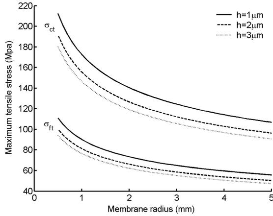
**Figure 5.** The maximum tensile stress of flat and corrugated membranes versus the membrane radius. (For the corrugated membrane,  $n = 5$ ,  $H:h = 10$ .)
