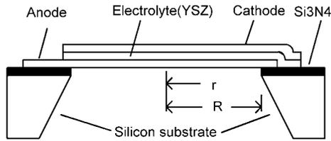
**Figure 1.** A schematic diagram of a thin film SOFC on silicon substrate.
