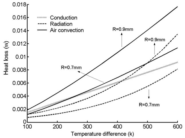
**Figure 11.** Heat loss versus temperature difference in a flat thin YSZ film with a less than 1 mm radius and  $3 \mu\text{m}$  thickness ( $T_b = 323 \text{ K}$ ).
