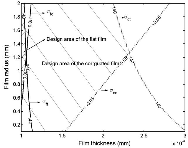
**Figure 7.** Design areas of corrugated films ( $H:h = 10:1$ ) and flat films under the buckling critical stress of 0.05 MPa and the fracture critical stress of 140 MPa.
