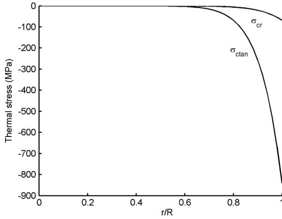
**Figure 8.** The radius and tangential thermal stress versus the relative membrane radius ( $H:h = 10:1$ ,  $\Delta T = 600^\circ\text{C}$ ).
