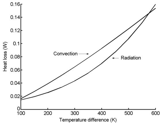
**Figure 13.** Heat loss versus temperature difference at the film radius of 3 mm.
