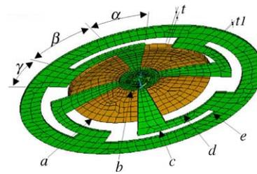
Fig. 3. Simulated bending mode of the actuating device. *t* and *a*: thickness and radius of the bimorph disc; *t*<sub>1</sub>, *c*, *d*: thickness, outer and inner radii of partial annulus of Z-tethers;  $\alpha$ ,  $\beta$ ,  $\gamma$ : angles of a sector and two partial annuli of Z-tethers; *b*: radius of the central poppet; *e*: inner radius of valve chamber.
