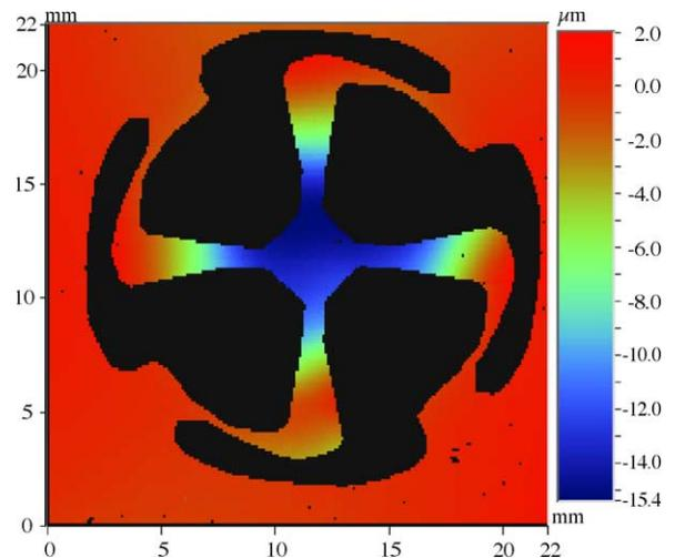
Fig. 9. Scanned 2D profile of the actuating diaphragm under 182 V voltage.
