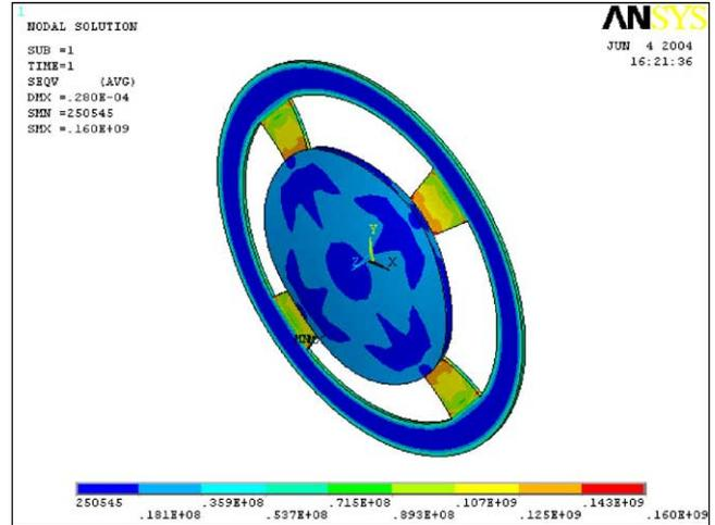
Fig. 5. Thermal deformation and stress distribution of an actuator with straight tethers at 120 °C.
