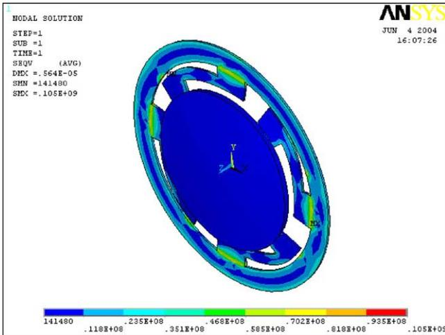
Fig. 4. Thermal deformation and stress distribution of an actuator with Z-tethers at 120 °C.
