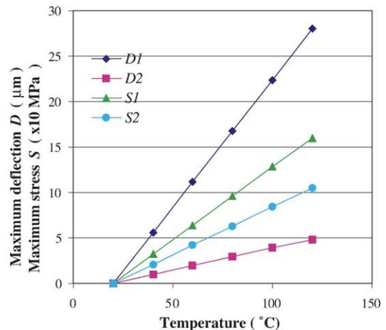
Fig. 6. Comparison of thermal deflection and stress of actuators with straight and Z-tethers.
