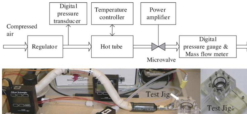
Fig. 11. Schematic and photograph of test setup.
