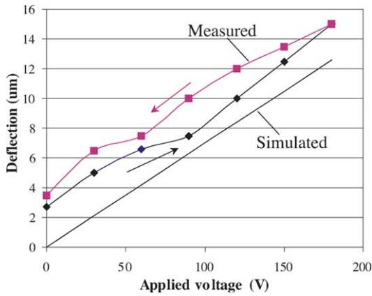
Fig. 10. Deflection in z-direction vs. applied voltage.
