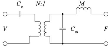
Fig. 7. Electromechanical equivalent circuit.  $C_e$  is the free electrical capacitance,  $N$  is the transducer ratio,  $C_m$  is compliance under open circuit conditions,  $V$  is the applied voltage,  $F$  is the applied force, and  $M$  is the effective mass.
