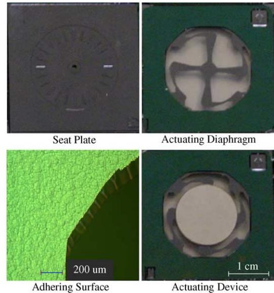
Fig. 8. Photograph of bulk-micromachined actuating diaphragm, bottom plate and actuating device.
