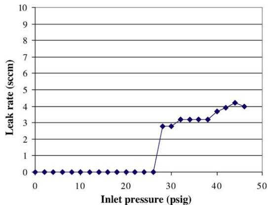
Fig. 14. Leak rate at inlet pressure up to 46 psig (room temperature).
