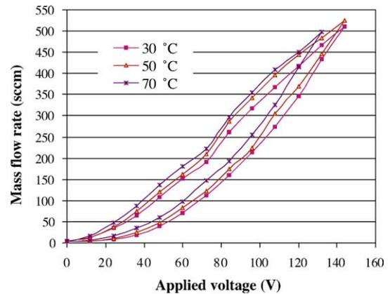
Fig. 13. Measured flow rate vs. applied voltage at different air temperature.
