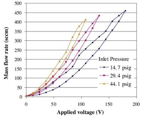
Fig. 12. Measured flow rate vs. applied voltage at different inlet pressure.
