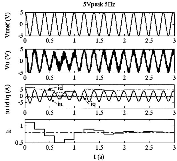
Fig. 5. Identifying compensation factor  $k$  by simulation.
