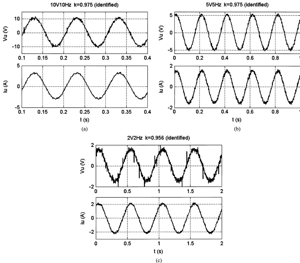
Fig. 9. Compensation results with identified compensation factor: (a) output with  $k = 0.975$  under  $10 V_{\text{peak}}$  10 Hz, (b) output with  $k = 0.975$  under  $5 V_{\text{peak}}$  5 Hz, and (c) output with  $k = 0.956$  under  $2 V_{\text{peak}}$  2 Hz.
