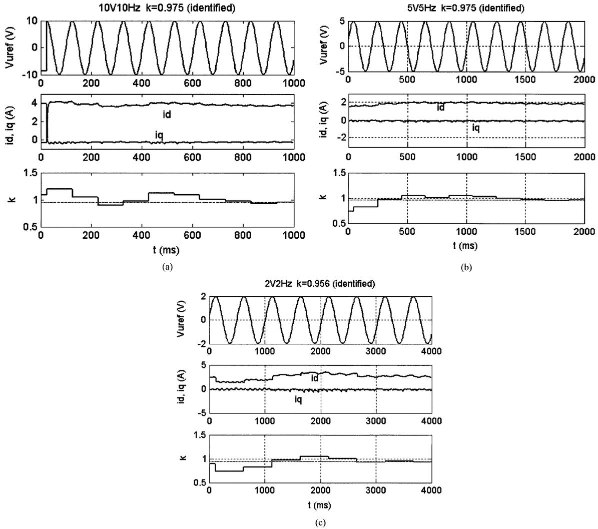
Fig. 8. Identification of compensation factor  $k$ : (a) identification under  $10 V_{\text{peak}}$  10 Hz, (b) identification under  $5 V_{\text{peak}}$  5 Hz, and (c) identification under  $2 V_{\text{peak}}$  2 Hz.
