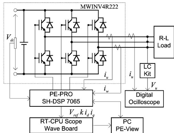
Fig. 7. Test system for identifying the compensation factor.
