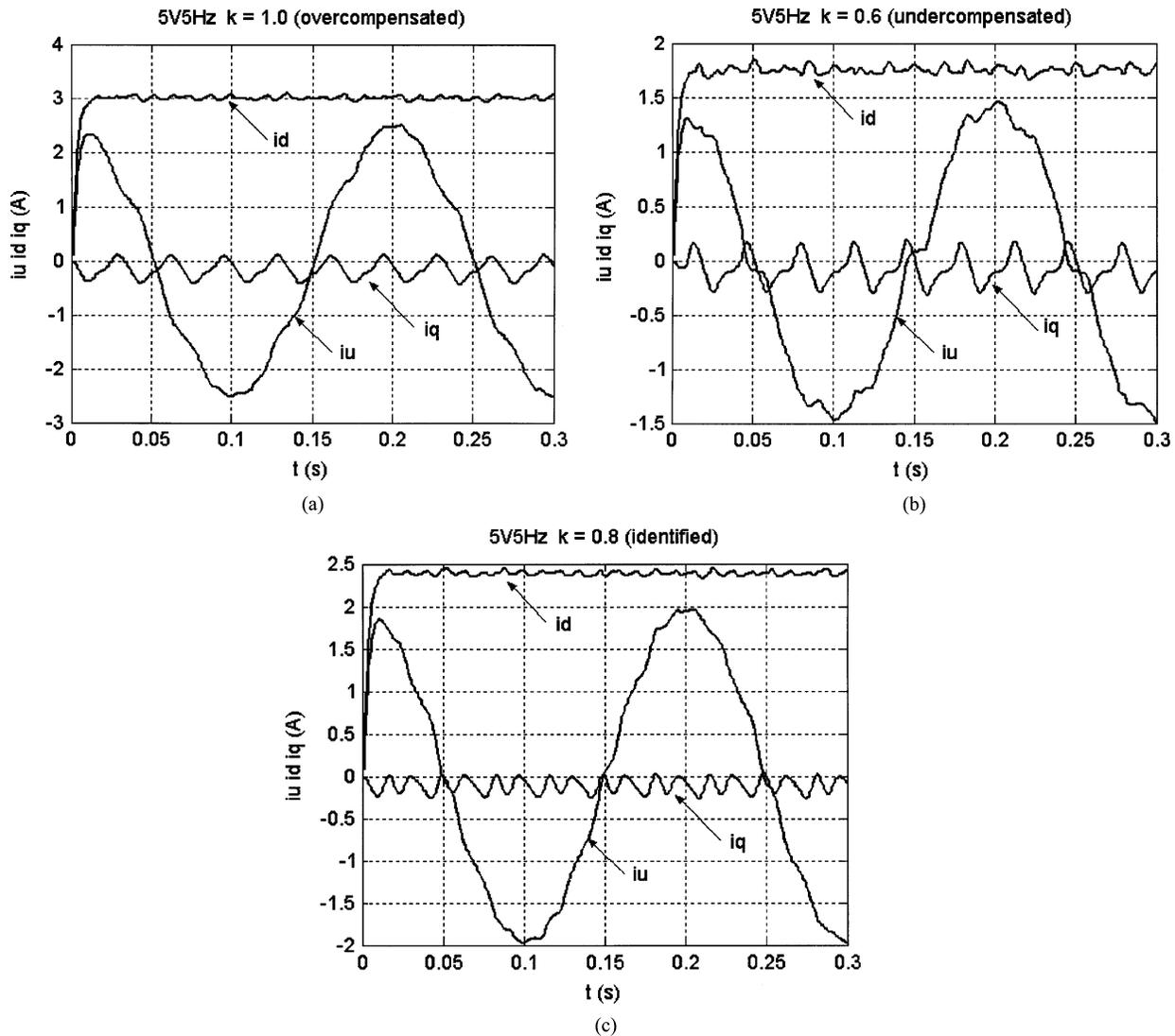
Fig. 6. Simulation results of compensation with  $k = 1.0$ ,  $0.6$ , and  $0.8$ : (a) overcompensation  $k = 1.0$ , (b) undercompensation  $k = 0.6$ , and (c) compensation with  $k = 0.8$ .
