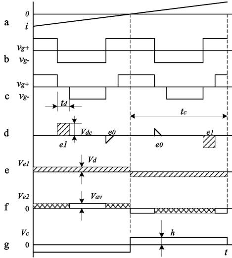
Fig. 2. Analysis of nonlinearity of VSI inverters: (a) phase current, (b) ideal gating pulses of the upper and lower switches of one leg, (c) actual gating pulse with the dead time  $t_d$ , (d) volt-second error during the dead time ( $e_1$ : caused by the switch,  $e_0$ : caused by the antiparallel diode), (e) average voltage error within one PWM period  $t_c$ , (f) constant voltage drop across the switch (blank area) and the diode (shaded area), and (g) compensation voltage.
