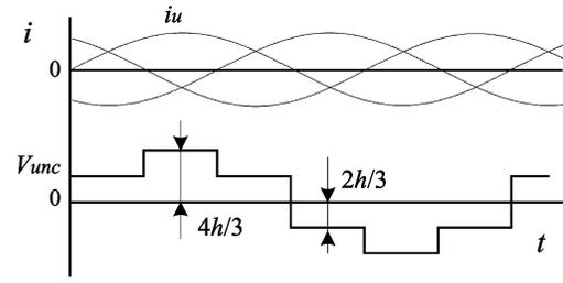
Fig. 3. Compensation voltage for one phase.
