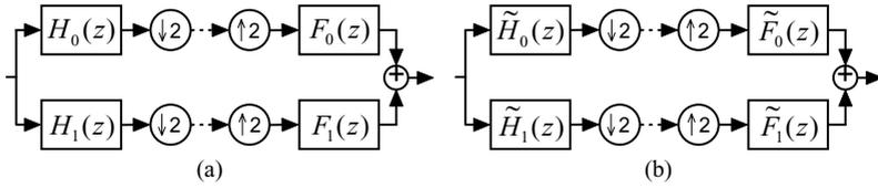
**Fig. 1.** (a) The primal filter bank  $\mathbf{B}$ ; (b) The dual filter bank  $\tilde{\mathbf{B}}$
