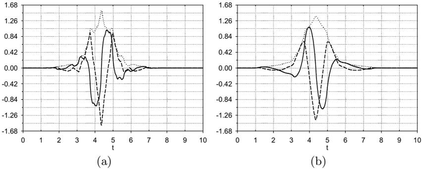
**Fig. 2.** Wavelets of the dual-tree complex filter bank 9/7–10/8. (a) Analysis side:  $\psi_h(t)$  (dashed line),  $\tilde{\psi}_h(t)$  (solid line), and  $|\psi_h(t) + j\tilde{\psi}_h(t)|$  (dotted line); (b) Synthesis side:  $\psi_f(t)$  (dashed line),  $\tilde{\psi}_f(t)$  (solid line), and  $|\psi_f(t) + j\tilde{\psi}_f(t)|$  (dotted line).
