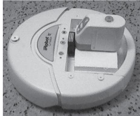
Fig. 2: The iRobot Create with the Virtual Wall mounted on it
