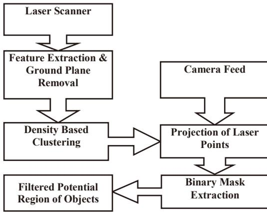
Fig. 1. Block Diagram of the Proposed Method.
