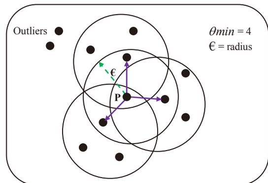
Fig. 3. An Example of DbSCAN Algorithm.
