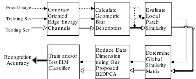
Fig. 2. Schematic diagram of our face recognition algorithm.
