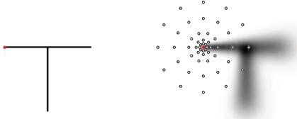
**Fig. 1.** A sparse signal  $S$  (left) and the geometric blur of  $S$  around the feature points marked in red [10].
