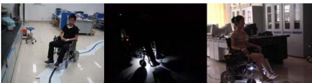
Figure 9. Visual navigation mode running in different light conditions
