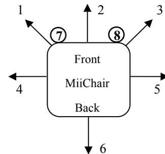
Figure 12. Distribution of ultrasonic sensors
