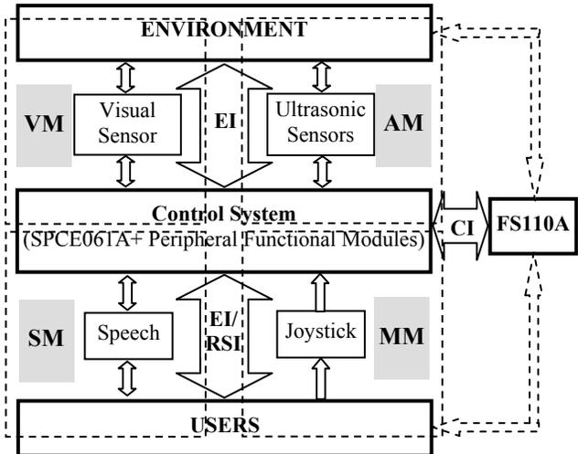
Figure 2. Structure of multi-mode embedded control system
