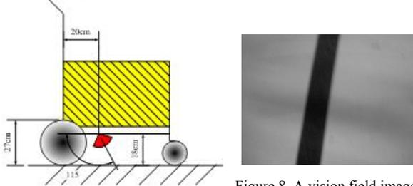
Figure 7. Position of visual sensor
