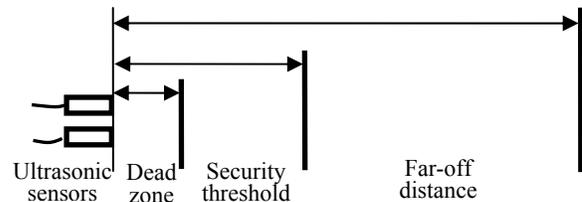
Figure 11. Distance measuring of ultrasonic sensors
