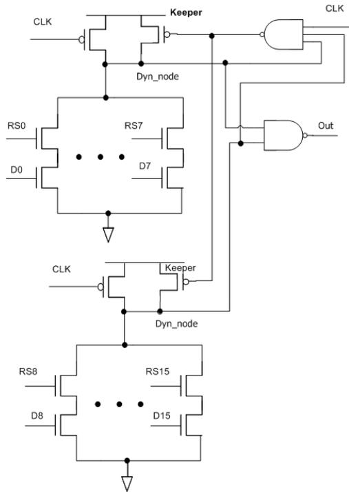
Figure 4 Split Domino technique with pull-down network split in two
