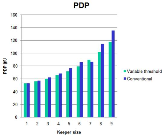
Figure 6 simulation results for variable threshold keeper technique for different keeper sizes
