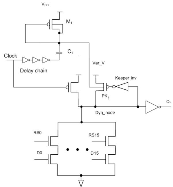
Figure 5 Variable-threshold keeper technique
