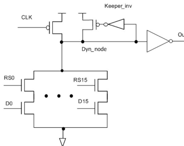
Figure 1 Multiplexer circuit with a conventional keeper
