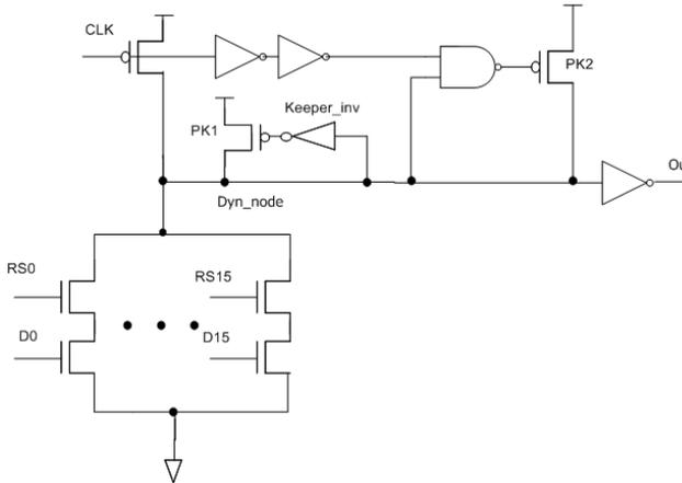
Figure 2 Dynamic logic with conditional keeper
