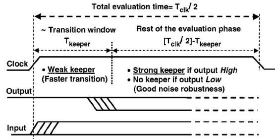
Figure 3 Conditional keeper timing diagram
