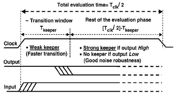
Figure 3 Conditional keeper timing diagram [5]
