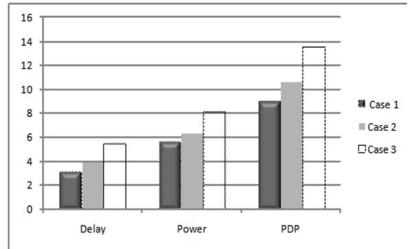
Figure 7 Proposed method performance improvement over conventional SD for three different delay constraints in percent
