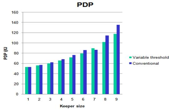
Figure 6 Simulation results for variable threshold keeper technique for different keeper sizes
