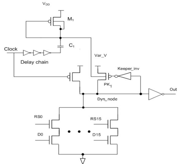
Figure 5 Variable Threshold keeper
