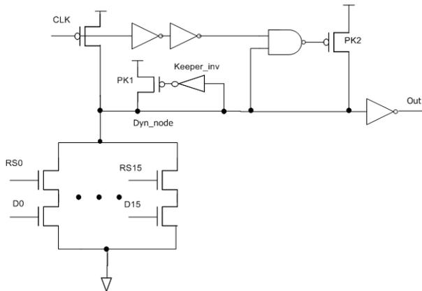
Figure 2 Dynamic logic with conditional keeper
