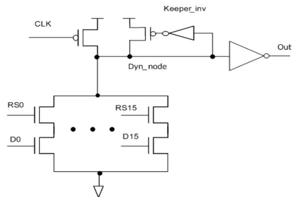
Figure 1 Multiplexer circuit with a conventional keeper
