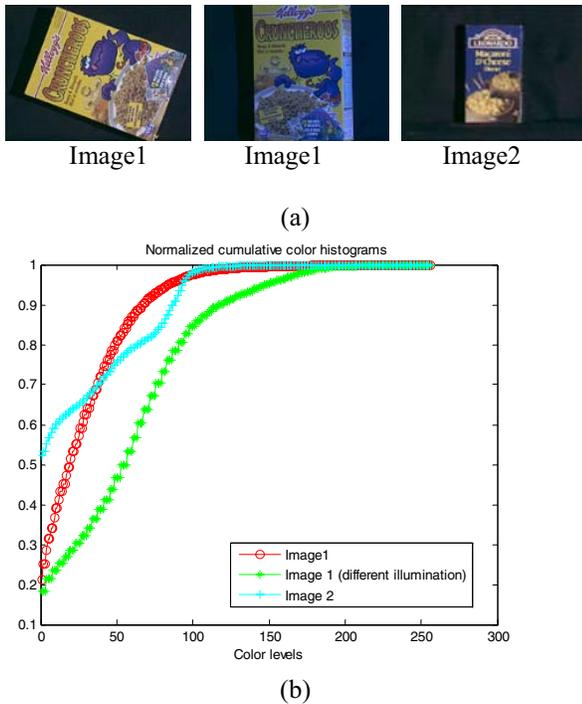
Figure 1. (a) Candidate images, Image 1, Image 1 with illumination change, and image 2; (b) Normalized cumulative colour histograms for the candidate images. It can be seen that the values are coarsely preserved for an object after illumination changes.
