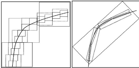
Figure 3. Edge representation using Wavelets (left) and Curvelets (right)
