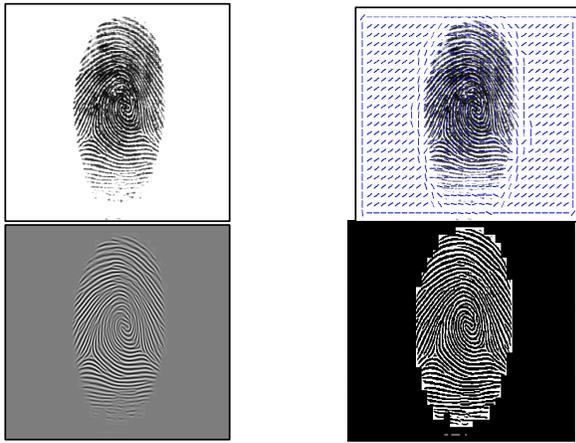
Figure 1. Top left: Original image, Top right: Ridge orientation detected image, Bottom left: Filtered image, Bottom right: Binarized image.
