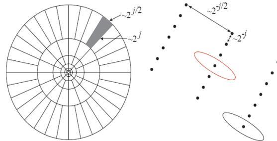
Figure 2. Curvelets in Fourier Frequency domain (left) and Spatial domain (right) [15]
