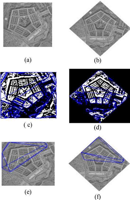
Figure 3. Partial convex hull information for image registration
