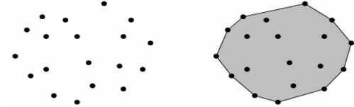
Figure. 1. Convex hull for a set of points in 2-D
