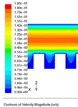
**Figure 7. Velocity field in the grooves**
