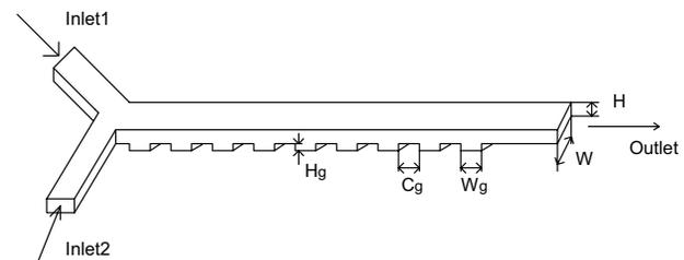
**Figure 1. Micromixer with patterned grooves, the angle between channel and grooves is 45°. The groove width  $W_g$  is equal to the distance  $C_g$  between adjacent grooves. The period of grooves  $Q$  is  $W_g + C_g$ .**
