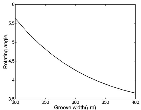
**Figure 8. Rotating angle versus groove width. Channel depth  $H$  is  $200\mu\text{m}$ , and groove depth  $H_g$  is  $50\mu\text{m}$ .**
