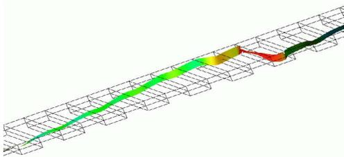
**Figure 3. Stretched and folded fluid streams in the channel with patterned grooves**
