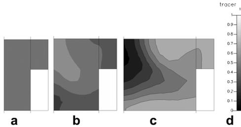
**Figure 6. Fluid2 fraction distributions in the cross section of the mixing channel. The channel width  $W$  is  $400\mu\text{m}$ . (a)  $H = 150\mu\text{m}$ ,  $\alpha = 3.67^\circ$ ,  $M = 0.99$  (b)  $H = 250\mu\text{m}$ ,  $\alpha = 1.59^\circ$ ,  $M = 0.84$  (c)  $H = 400\mu\text{m}$ ,  $\alpha = 0.47^\circ$   $M = 0.65$**
