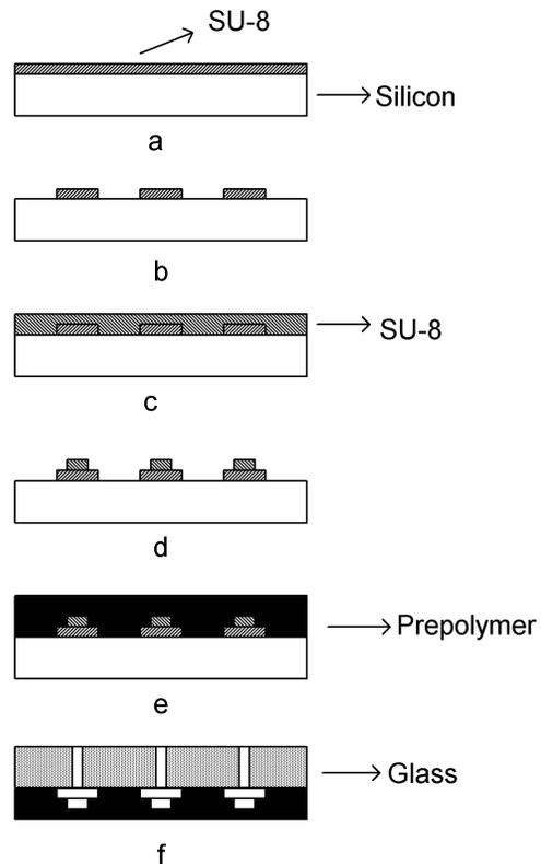
**Figure 10. Fabrication process of replica molding of micromixer. (a) The first SU-8 layer is coated on the silicon substrate. (b) The channel pattern is transferred to SU-8. (c) The second SU-8 layer is coated on the silicon substrate. (d) The groove pattern is transferred to the second SU-8 layer. (e) Prepolymer is cast to the SU-8 mold. (f) Cured PDMS is bonded to glass.**
