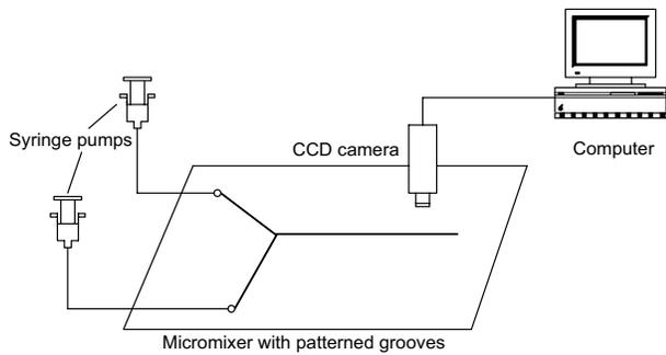
**Figure 11. Schematic setup for mixing experiments**
