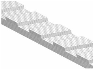
**Figure 2. Meshed channel and grooves**
