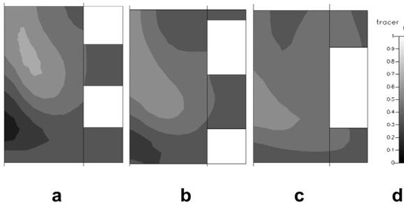
**Figure 9. Fluid2 fraction distributions in the cross section of the mixing channel. The groove depth  $H_g$  is  $100 \mu\text{m}$  (a)  $W_g = 50 \mu\text{m}$ ,  $\alpha = 0.67^\circ$ ,  $M = 0.75$  (b)  $W_g = 100 \mu\text{m}$ ,  $\alpha = 1.94^\circ$ ,  $M = 0.80$  (c)  $W_g = 150 \mu\text{m}$ ,  $\alpha = 2.18^\circ$ ,  $M = 0.90$ .**
