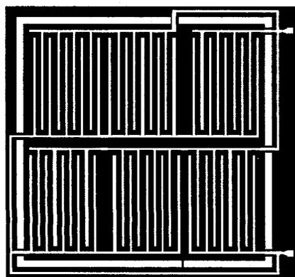
Figure 4: Interdigitated etch mask
