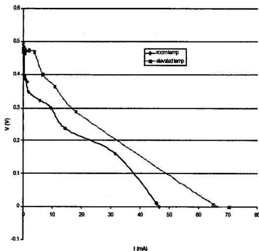
**Figure 11: Voltage-Current Characteristics**
