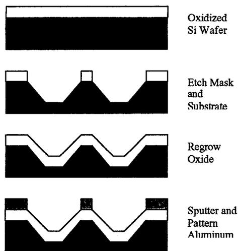
Figure 3: Fabrication process
