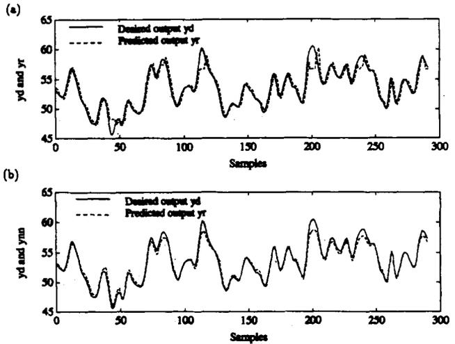
Figure 2: The desired output and the output predicted by the fuzzy model. a) Without the NN compensator. b) With the NN compensator.
